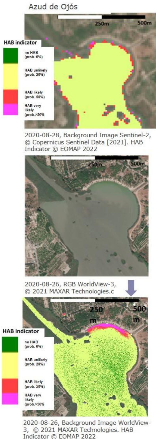
Figure 1. HAB indicator by utilizing different spaceborne images (i.e., Sentinel-2 (top) vs. WorldView-3 (bottom)).
